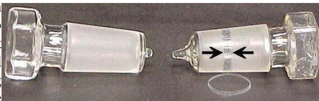
Figure 3: Press-Fit-Mechanism of PTFE Sealing Ring (Glindemann)
